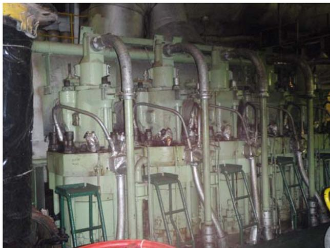
Reduced load primarily results in increased carbonisation and low temperature corrosion. Reduced load will also affect the combustion system, and lead to poor atomisation of the fuel nozzles.
