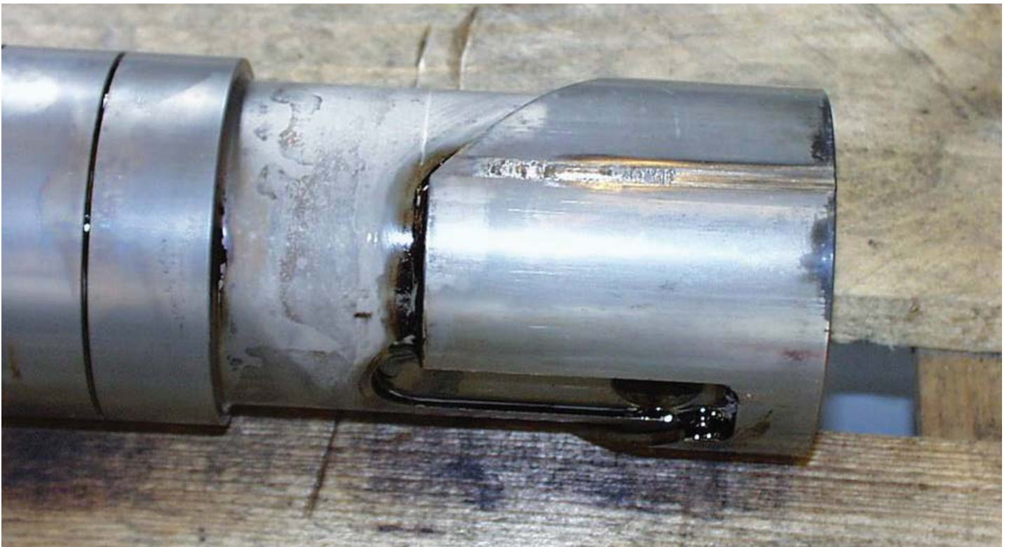
Fig. 7: Fuel pump plunger sticking
