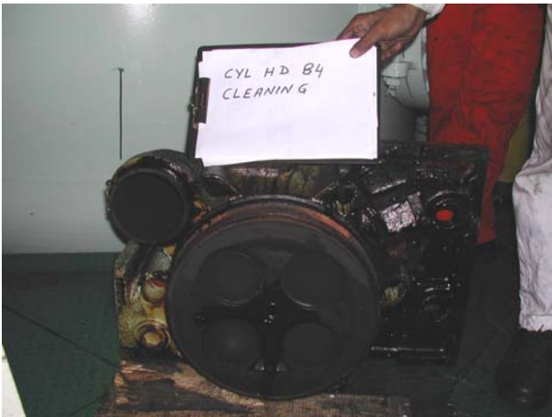
Fig. 2: Cylinder head cleaning
