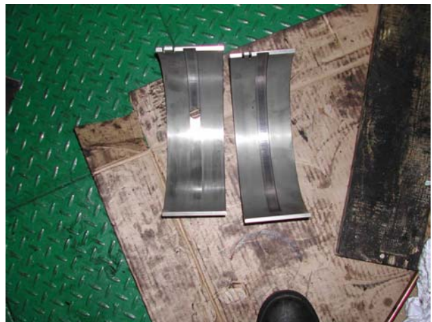
Fig. 15: Connecting rod bottom-end bearing dismantled and cleaned before dye checking.
